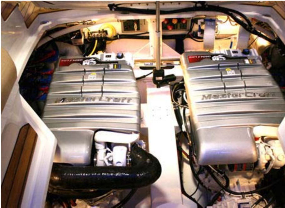
Twin 350-hp Indmar V-drives are easy to access from the helm area.
